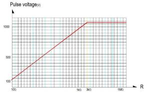
Pulse load rating in accordance with IEC 60115-1,4.27; 10 $\mu$ s/700 $\mu$ s; 10 pulses loaded, for permissible resistance change <±(0.5%+0.05 $\Omega$ )
