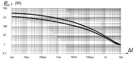
Maximum pulse load, single pulse; applicable if  $P \rightarrow 0$  and n≤1000 and  $\hat{U} \leq 4kV$ ; for permissible resistance change equivalent to 8000h operation in power operation mode.
